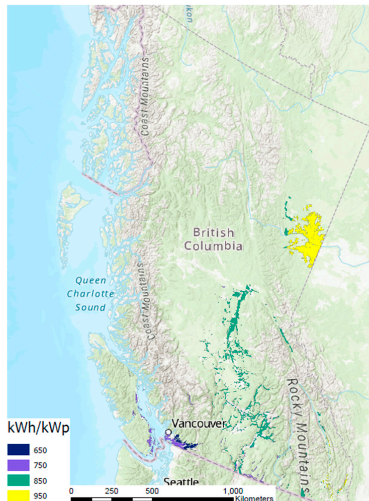
Figure 8. Conventional photovoltaic potential (in kWh/kWp) of south-facing, vertically oriented arrays in the farmland regions across British Columbia [97,98,104].
